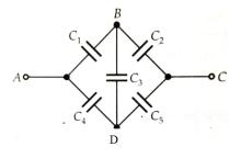
As  $C_1 = C_2 = C_4 = C_5$ Therefore,  $\frac{C_1}{C_2} = \frac{C_4}{C_5}$
